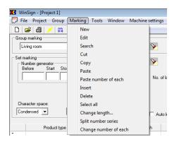
Above you see the marking menu (extended) and also a project window. The lower line of icons belongs to the marking section of the project.
